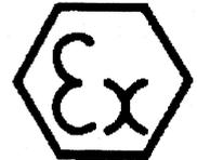
2 **Component intended for use in Potentially Explosive Atmospheres - Directive 94/9/EC**
